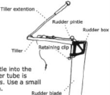
Warning - never force the rudder pintle into the sternpost, and make sure that the rudder tube is free of sand and is lubricated at all times. Use a small amount of grease, oil or even sunscreen.
